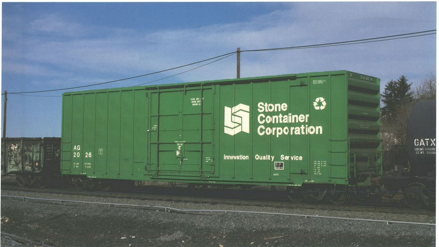
AG 2026. Built 7-90 GUX P. 5757 cubic foot capacity. Photographed March 28, 1991 in Hagerstown, MD. Kenneth Lehman.
