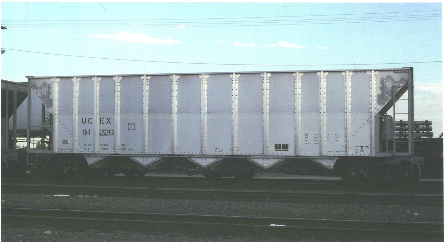
UCEX 91220. Built 4-91 TRN MO. 4000 cubic foot capacity. Photographed at Cheyenne, WY on June 28, 1991. T.E. Cobb.
