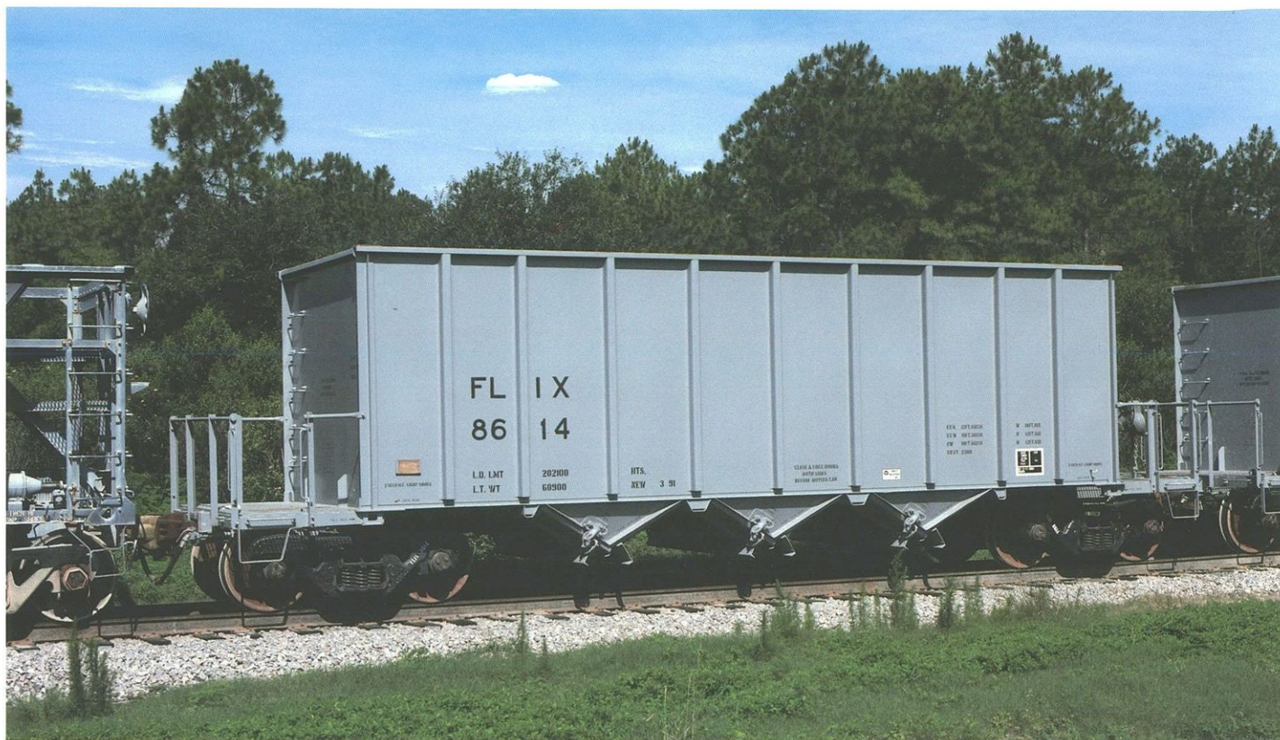
FLIX 8614. 202 HTS Built 3-91 TRN FWS. 2300 cubic foot capacity. Photographed June 1991 south of Mulberry, FL. D.G. Casdorph.
