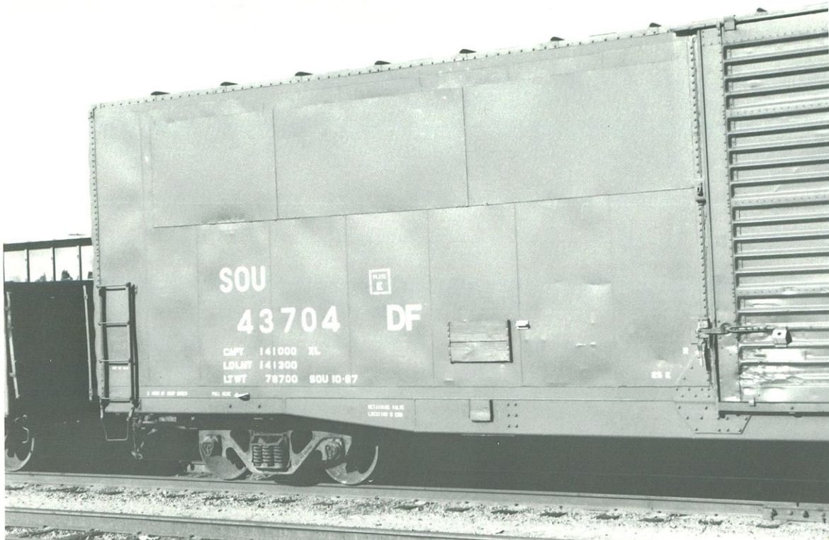
SOU 43704 is an interior post, "smoothside" box car. The repair panels are obvious and again can be made by using thin sheet styrene simply glued over the existing car side and then airbrushing the entire car.
