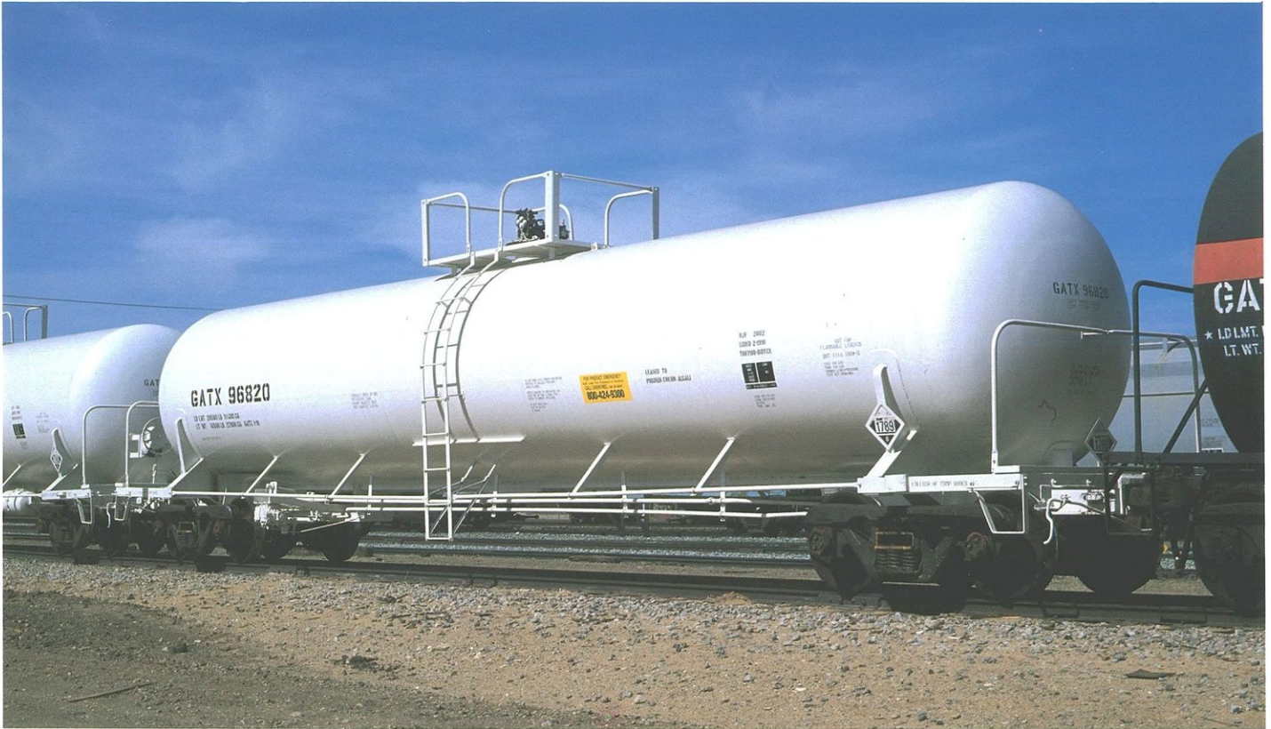
GATX 96820. Converted 1-91 to a DOT class 111A100W5. Leased to Pioneer Chloralkali. Photographed in May 1991 at Mojave, CA on the new Fuji Velvia (ISO 50) slide film. Note how white the whites are! D.G. Casdorph.
