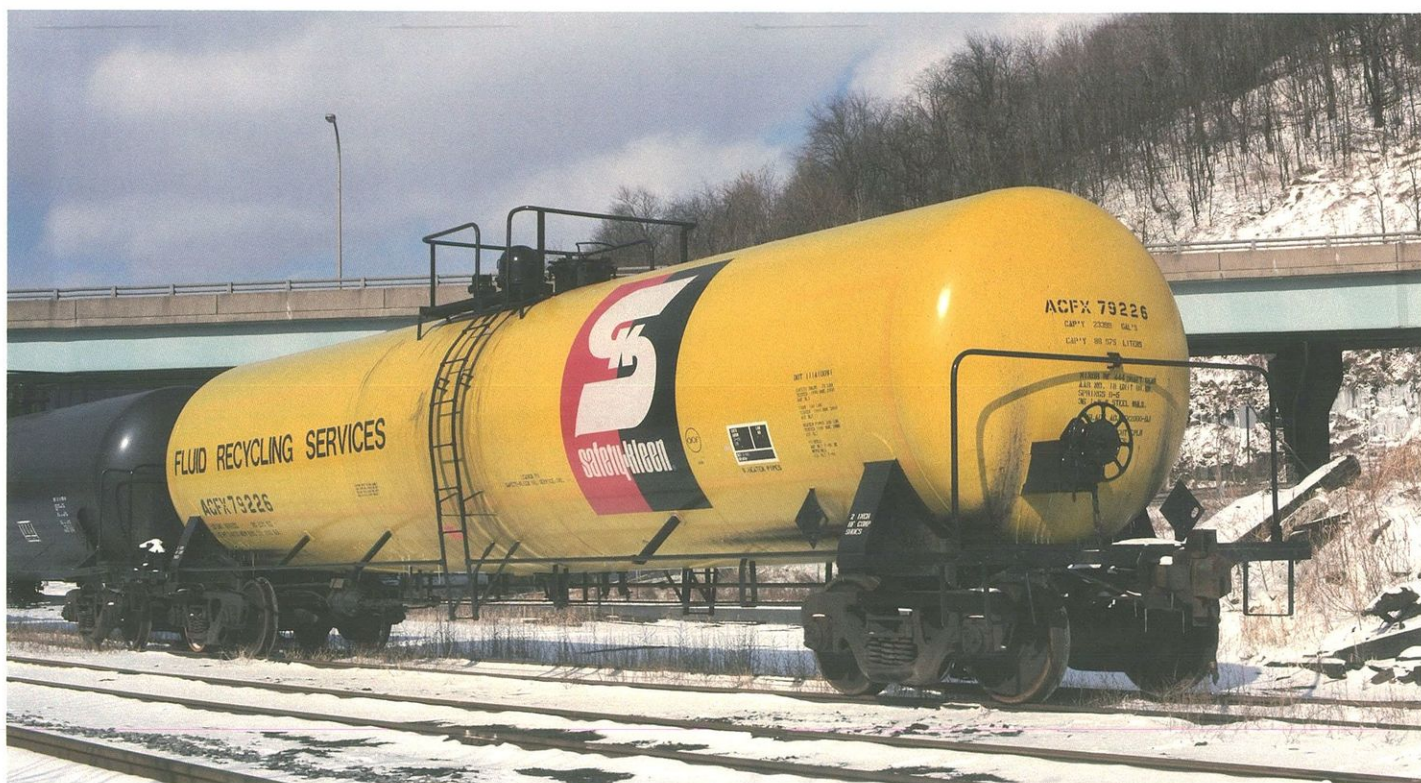
ACFX 79226. Painted 7-90 ACF MILT. Built 2-80 ACF MILT. Safety-Kleen Oil Service, Inc. Tank is non-insulated and has heater coils. 23,399 gallon capacity. Feb. 16, 1991. Johnstown, PA. Kenneth Lehman photo.
