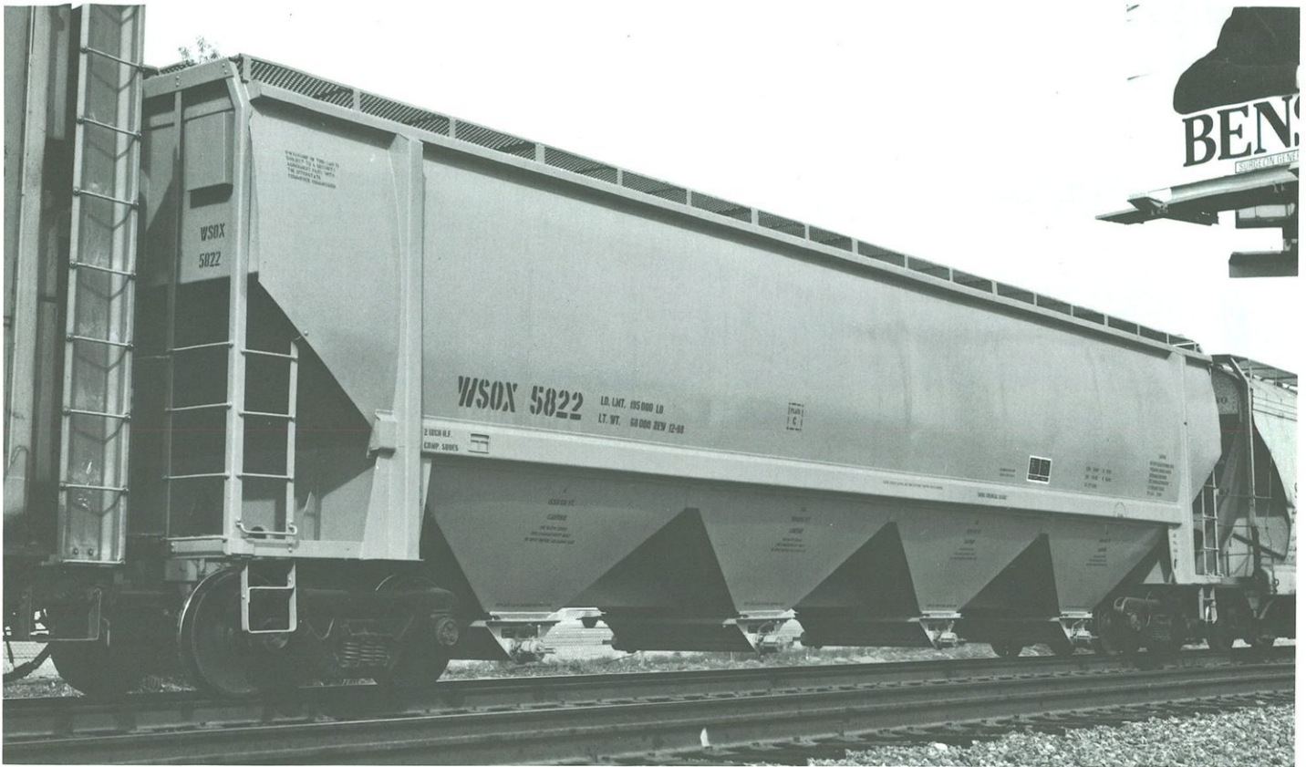
WSOX 5822 was built in 12-88 by Gulf Railcar. Its the same design as the Richmond Tank Car design introduced in the early 1980s. Note the massive exterior frame, rounded sides and exposed hoppers.
