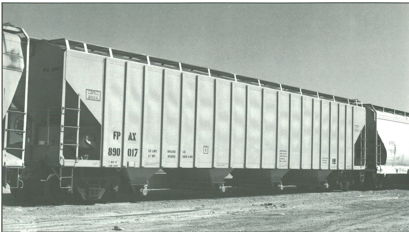
FPAX 890017 is a Trinity 5850 design. It evolved from the earlier PS 5820 (see PTLX 41519). This car was built in 6-89.
