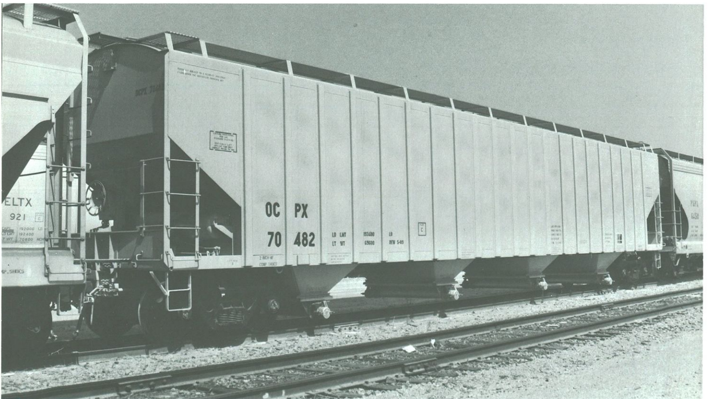
OCPX 70482 is Trinity's 6150 design. Note the height of the hopper area on the ends compared to the PS 5820 and TRN 5850 designs.
