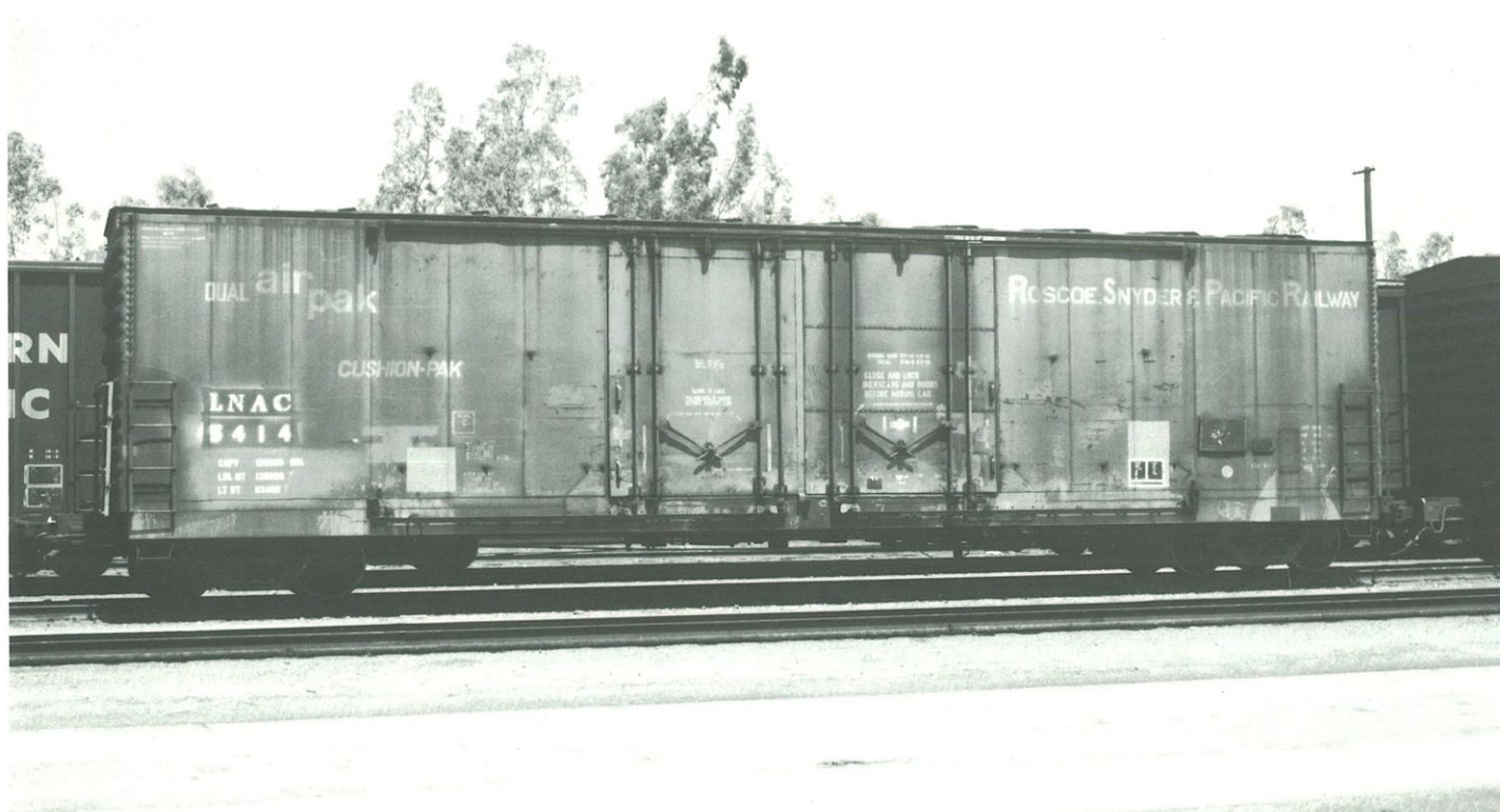
LNAC 5414 was built in 5-71 as part of the Roscoe, Snyder & Pacific 2000-series. Note the slightly different doors. Also, look at how sharp the original lettering (logos, etc.) is compared to the repainted reporting mark and number.
