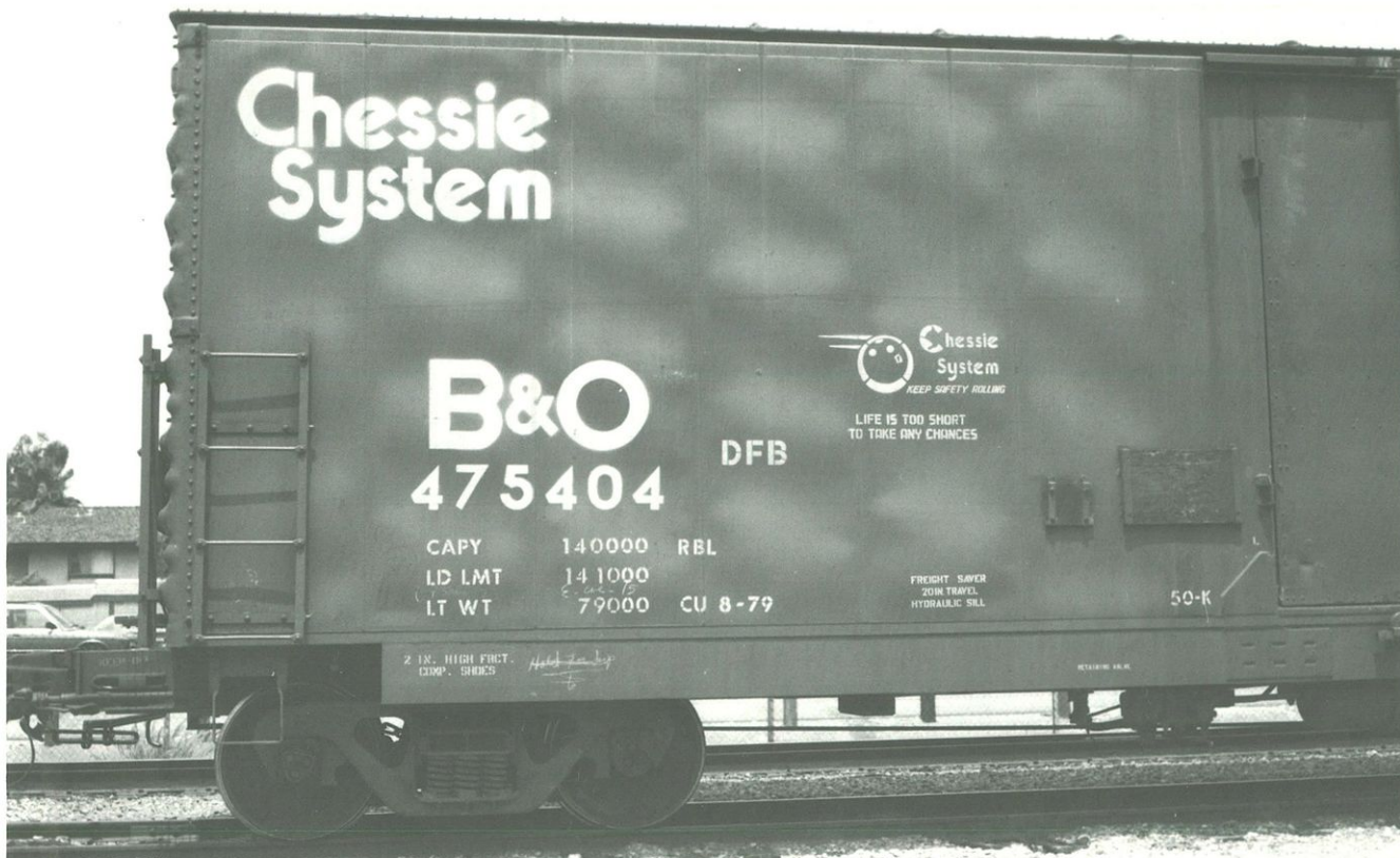
B&O 475404 left side. Note the Chessie "keep safety rolling" ball and slogan. Note that the ladders have been cut off about halfway on this end.
