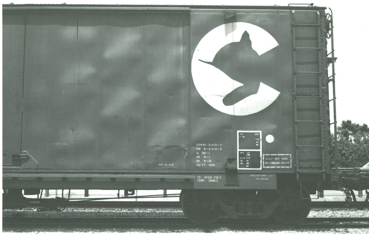
B&O 475404 right side. Note the original full height ladders, high mounted handbrake wheel and stenciled warning to keep on roof.
