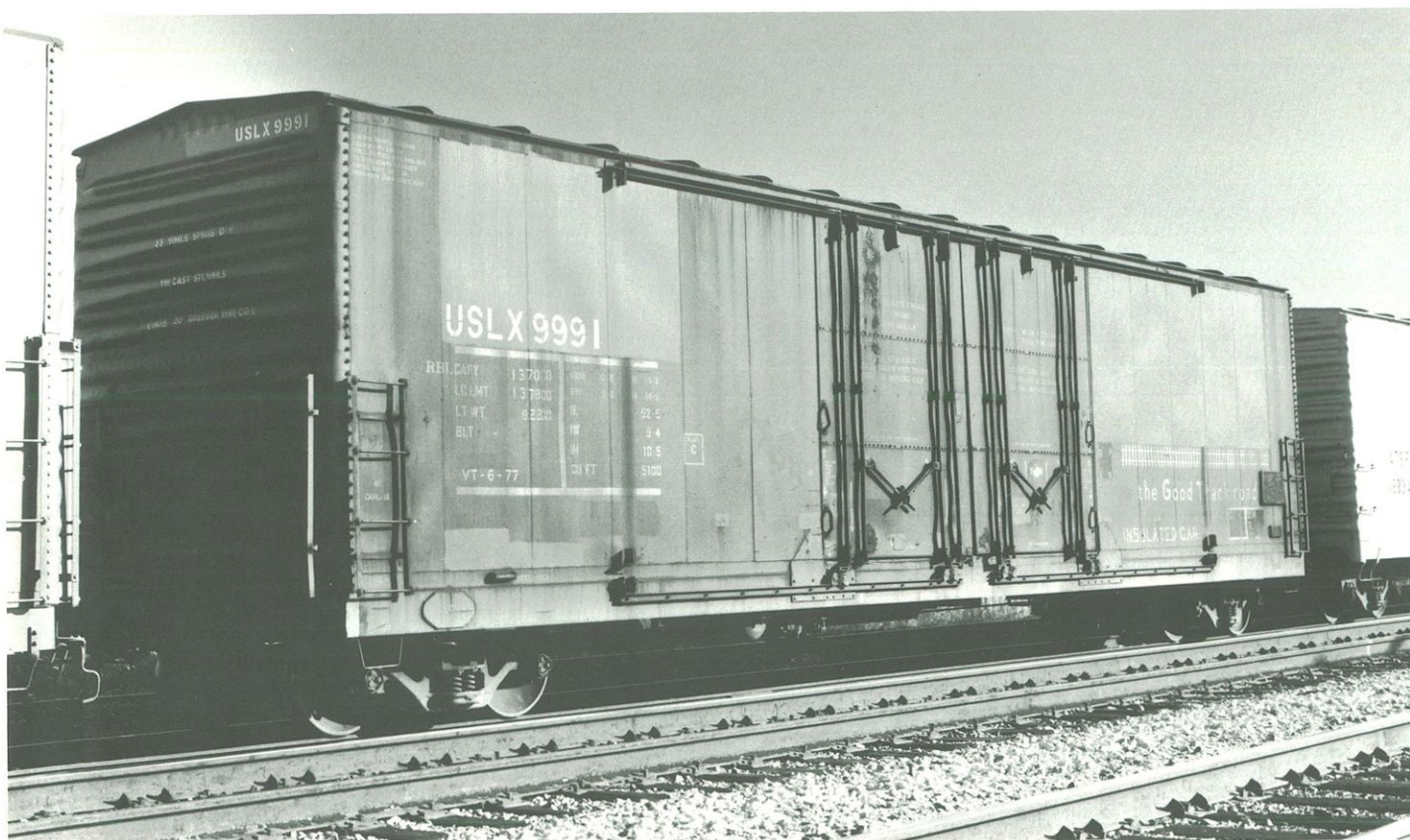
USLX 9991. Originally built for the Grand Trunk Western in 9-69. It was painted at the Port Huron Shops in 6-77. Relettered sometime in 1988 into USLX reporting mark and number.
