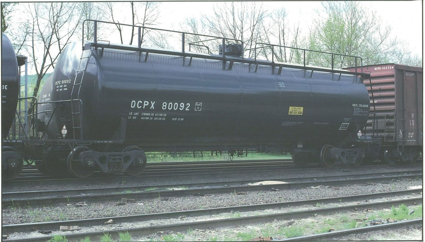
OCPX 80092. Built in 12-90 by Trinity for vinyl chloride transport. Note the full length top walkway. Photographed in May 1991 at Allentown, PA. E. A. Neubauer photo.
