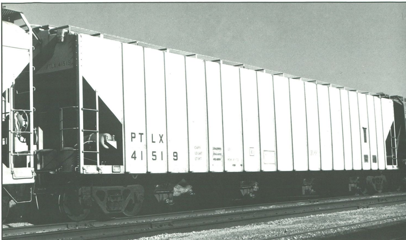
PTLX 41519. Built in 10-72. This is Pullman-Standard's 5820 design with rectangular body, exterior ribs etc.
